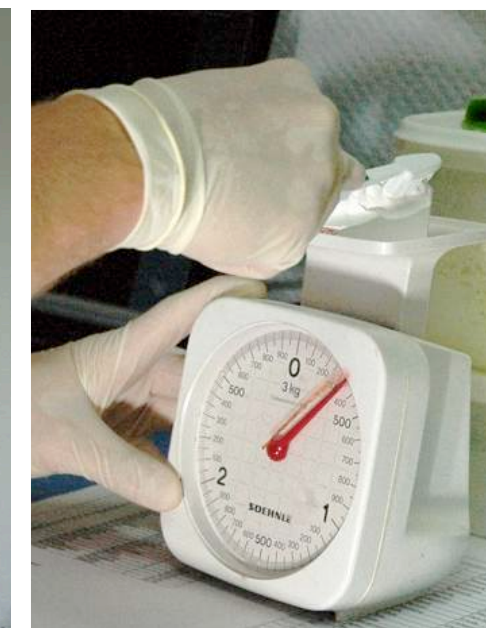
Calibration of brushing pressure to 3.5 N
